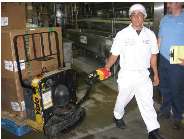
Pulling electric pallet jack.
